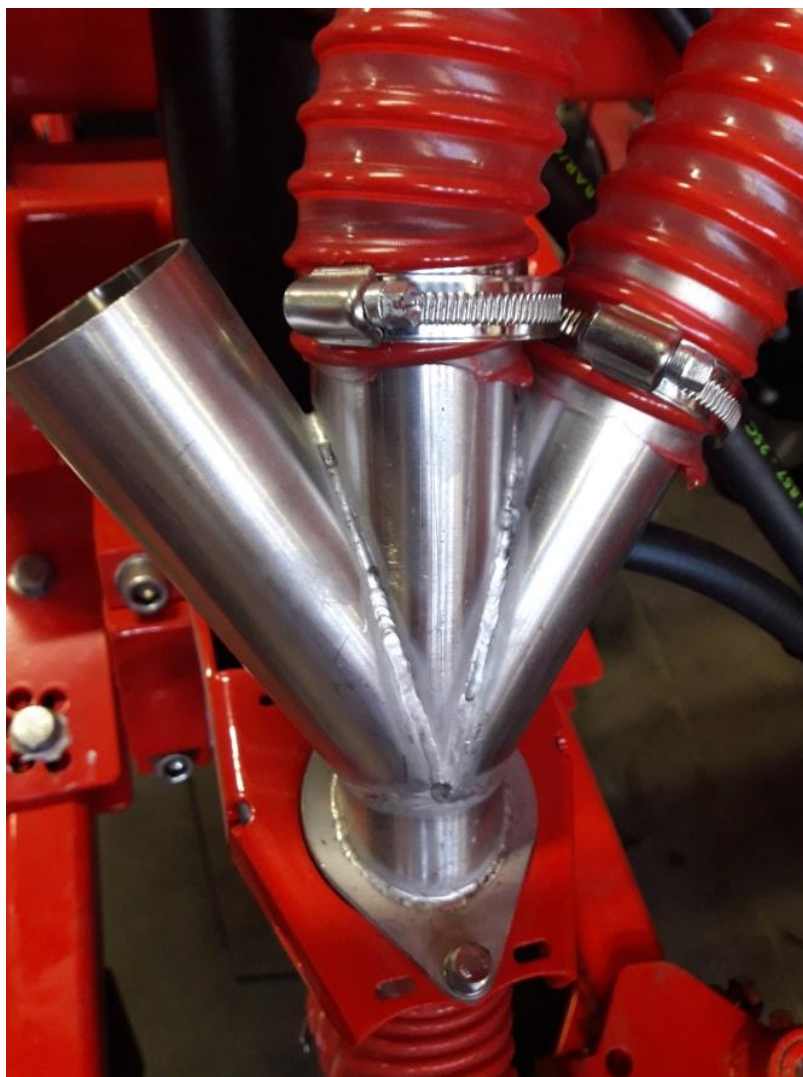
Fig. 67. Connecting the fertilizer hoses to the distributor of the working section
