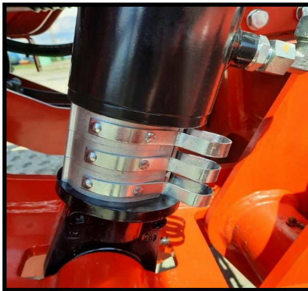
Fig. 77. Securing clips on hydraulic cylinders
