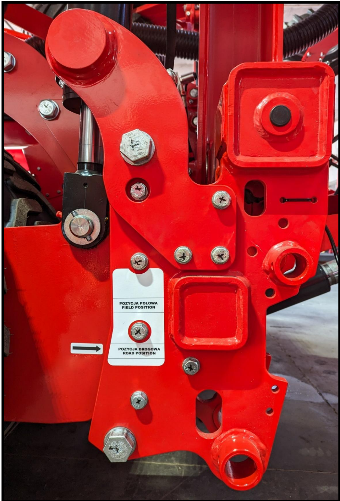
Fig. 54. Shock absorption system in road position
