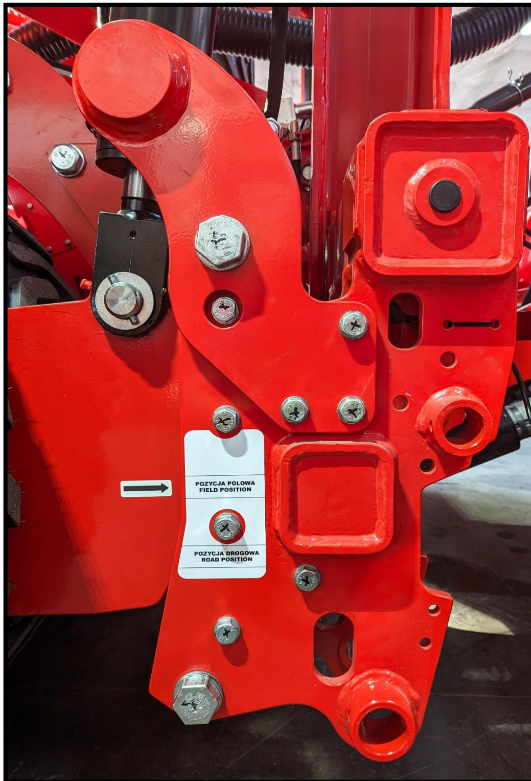
Fig. 53. Shock absorption system in field position
