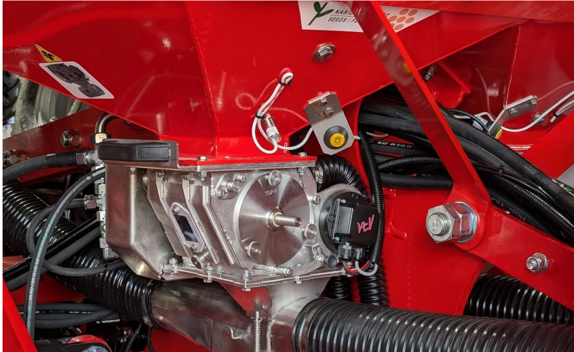
Fig. 63. Seeding device calibration test button placement
